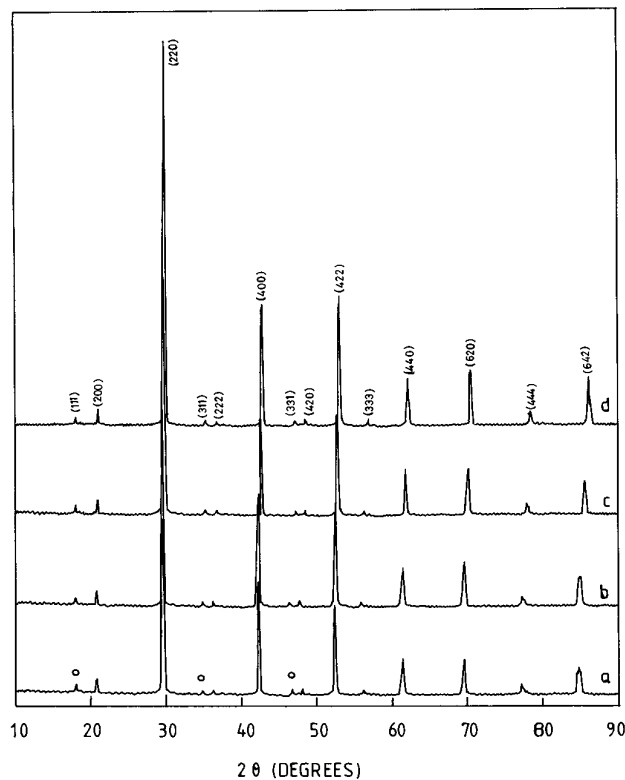
FIG. 1. X-ray diffraction patterns of sintered (a) Ba 2 PrTaO 6 , (b) Ba 2 NdTaO 6 , (c) Ba 2 EuTaO 6 , and (d) Ba 2 DyTaO 6 compounds. The superstructure lines are marked by 'o'.
